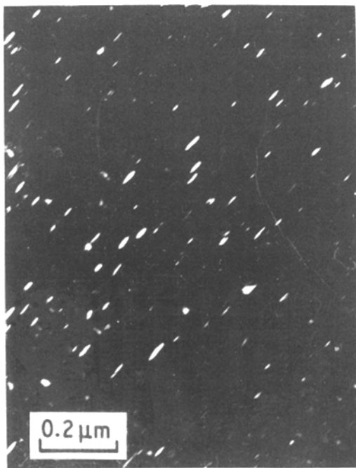
Figure 11 Dark-field micrograph obtained for Alloy 1, aged for 120 h at 450° C.
